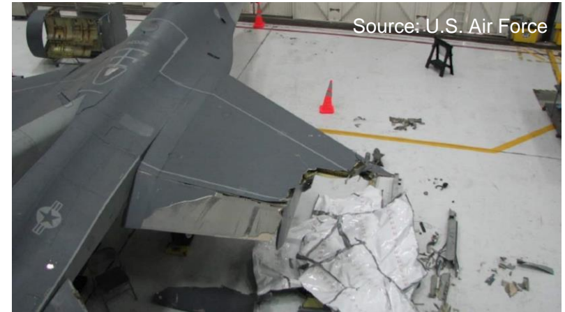
Example 1: F-16 with damaged wing.
