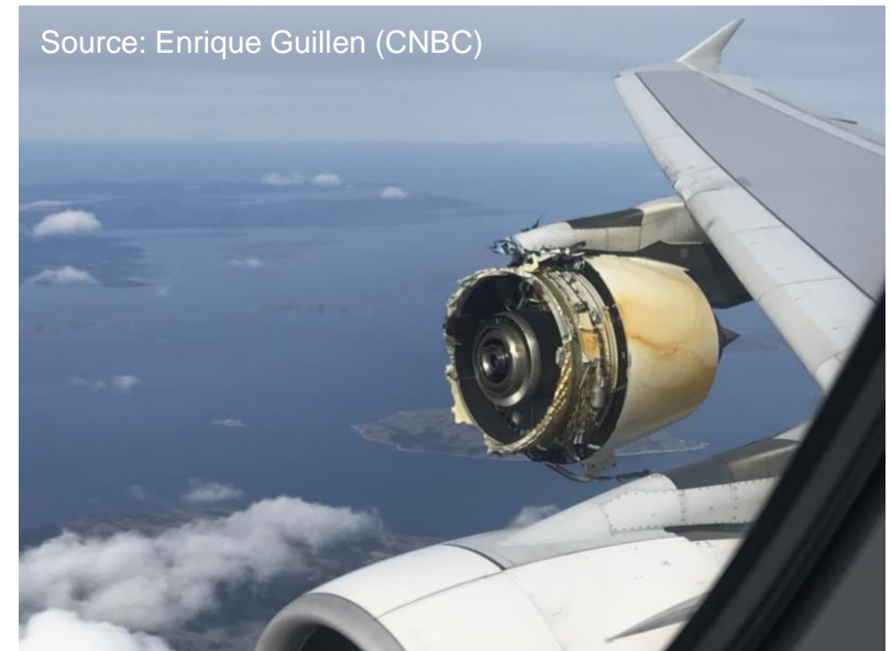
Example 2: Airbus A380 with engine failure.
